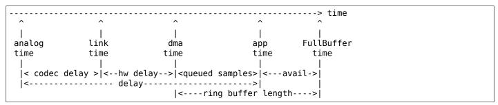
The analog time is taken at the last stage of the playback, as close as possible to the actual transducer
